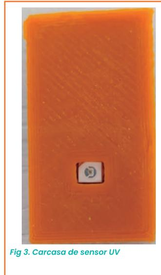
Fig 3. Carcasa de sensor UV
